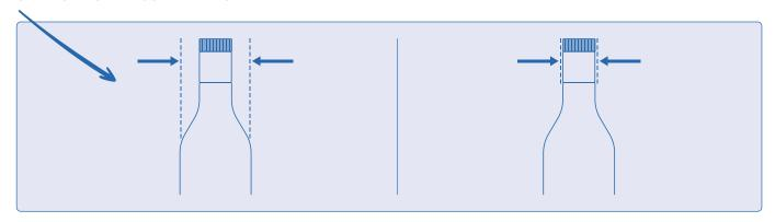
Measure the widest point over which the seal must pass, then add 1mm. For example, if the diameter of the cap is 50mm you would choose a seal of 51mm diameter.
